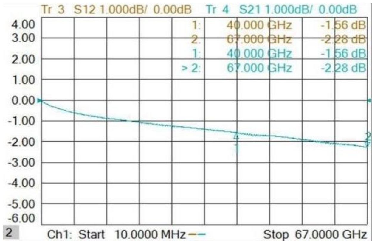
Figure 9 - Cable Loss Over Frequency
