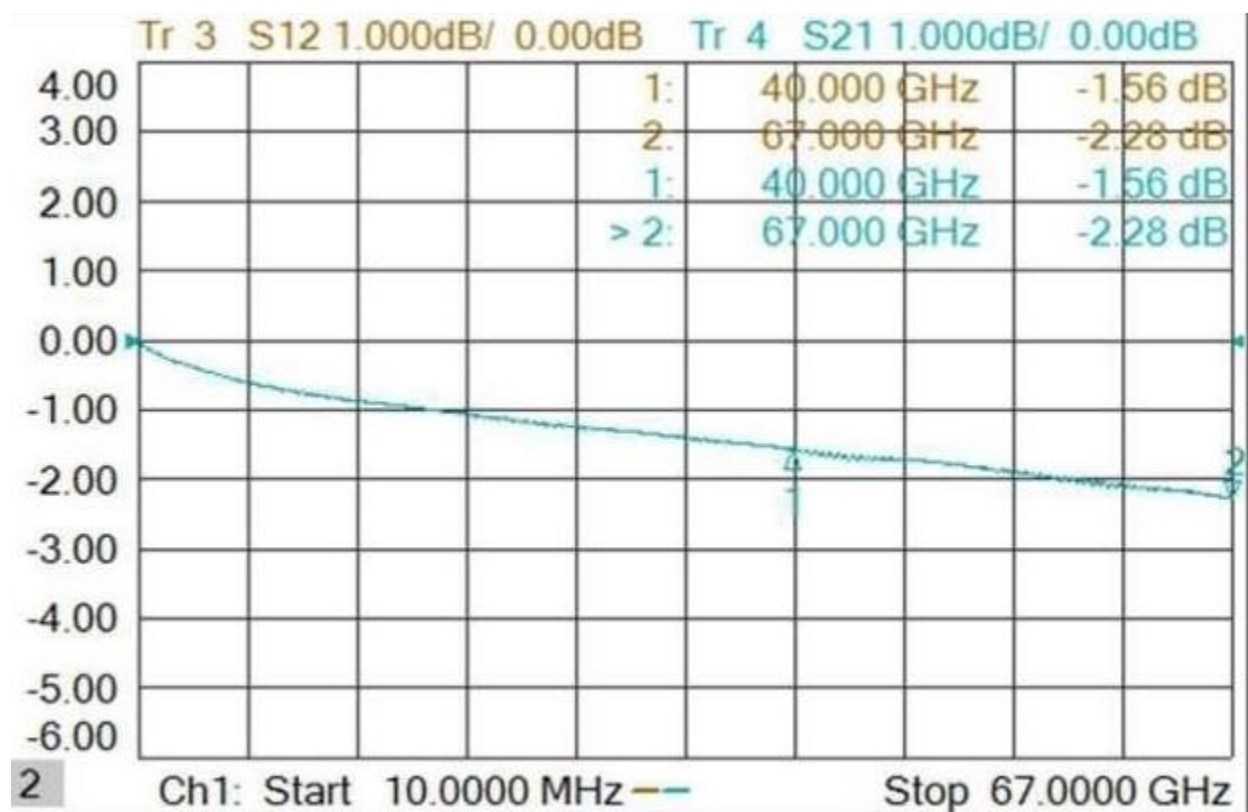
Figure 5 - Cable Loss Over Frequency
